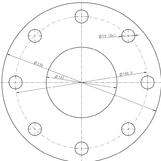
If a customer process flange with an inner diameter of more than 4" (101.6 mm) or an unsuitable gasket is used the flange joint will become leak-prone.
