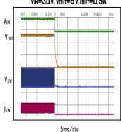
Switching Waveform V<sub>IN</sub>=12 V, V<sub>OUT</sub>=5 V, I<sub>OUT</sub>=0.1A
