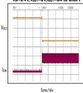
Short-Circuit Recovery VIN=24V, VOUT=5V, IOUT= Short to OA
