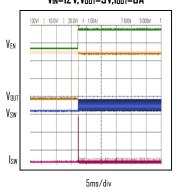
Start-up Waveform with EN=V<sub>IN</sub> V<sub>IN</sub>=12 V, V<sub>OUT</sub>=5 V, I<sub>OUT</sub>=0 A
