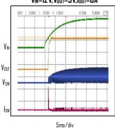
Shutdown Waveform with EN V<sub>IN</sub>=30V, V<sub>OUT</sub>=5V, I<sub>OUT</sub>=0.5A
