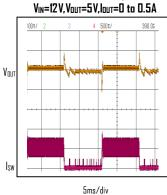
Short-Circuit Response V<sub>IN</sub>=24V,V<sub>OUT</sub>=5V,I<sub>OUT</sub>=0A to Short
