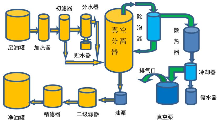
(废油罐 Used oil tank, 加热器 Heater, 初滤器 Pre-filter, 分水器 Water separator, 贮水器 Water receiver, 真空分离器 Vacuum separation tank, 油泵 Oil pump, 油泵 Oil pump, 二级滤器 Secondary filter, 精滤器 Fine filter, 净油罐 Clean oil tank, 除泡器 Foam breaker, 散热器 Radiator, 储水器 Water receiver, 真空泵 Vacuum pump, 冷却器 Cooler, 储水器 Water receiver, 排气口 Exhaust port.)
