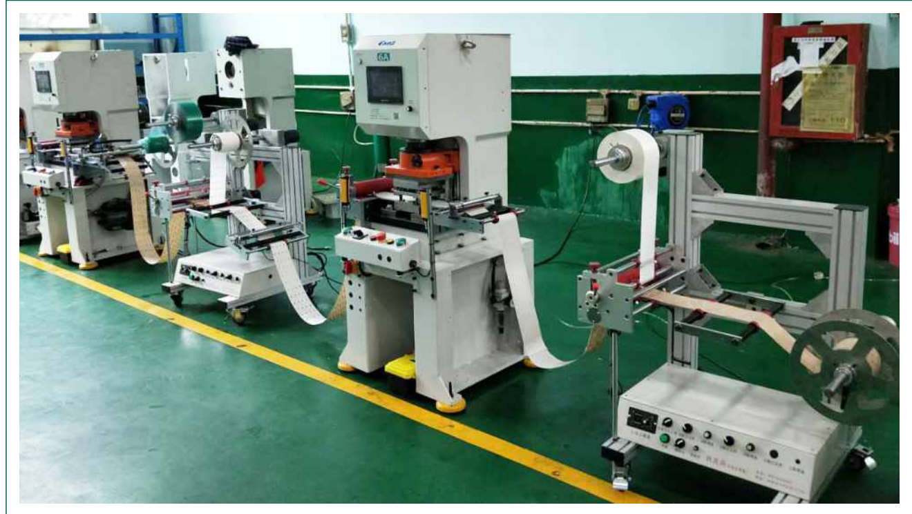
针对卷状材料（金属或非金属）二次套位冲压成型 Stamping forming of coil material (metal or non-metal) two times.
