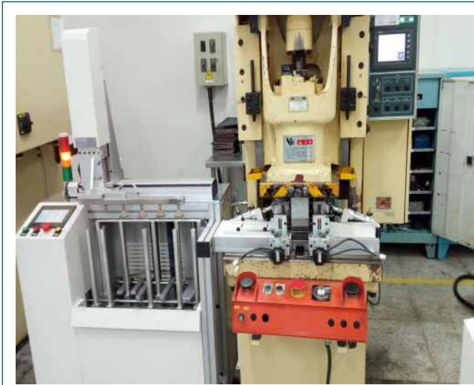
针对片状材料（金属或非金属）进行全自动连续冲压成型 For sheet materials (metals or nonmetals) Automatic continuous stamping forming.
