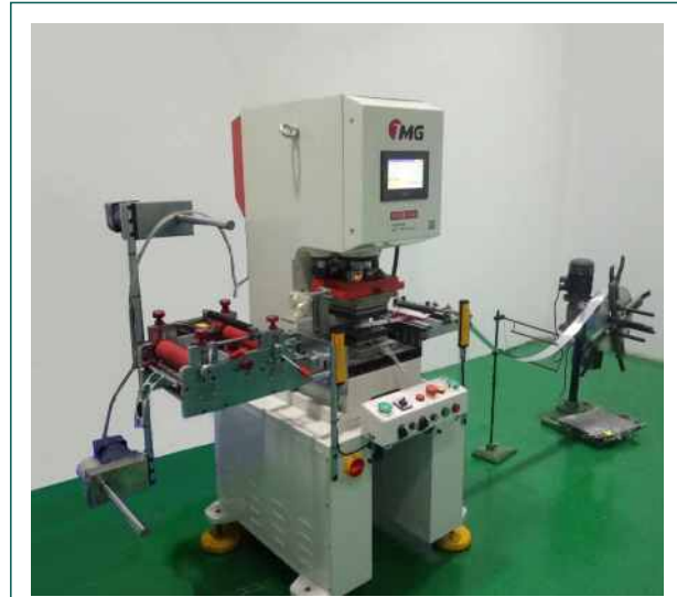
针对卷状材料金属拉伸或非金属凸包进行自动化作业 Automatic operation of metal drawing or non-metallic convex hull for coil material
