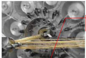
4.7 Pultrusion Pull-winding machine
