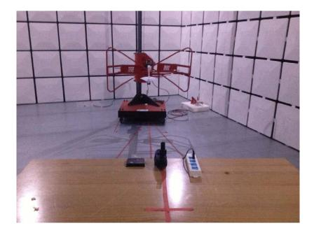
Radiated emission test setup photographs
